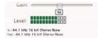
Gain Level set to optimum value. Well balanced audio with little or no distortion should be captured.
