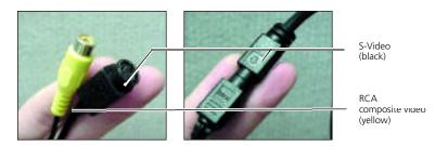
• Using the video extension cable that came with your camcorder, VCR or tuner, connect either the composite RCA (yellow) connector or the S-video (black)connector
